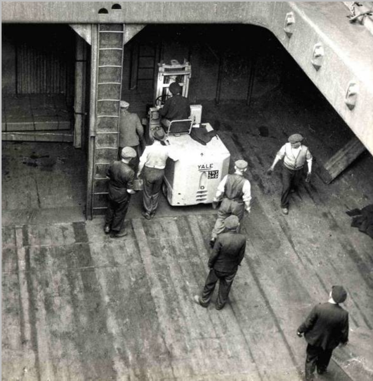
Fork lift truck stowing bundles of steel sheets under deck.
