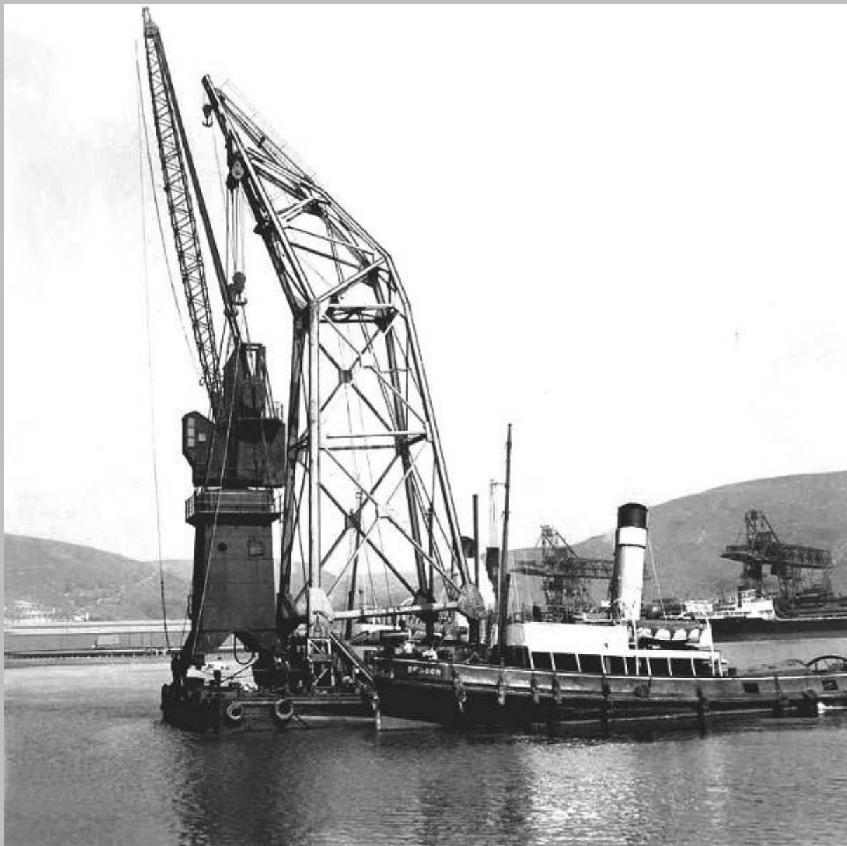
100 ton floating crane carrying hydraulic quayside crane across Port Talbot Dock – tugs 'Benson' & 'Herculaneum' 1960
