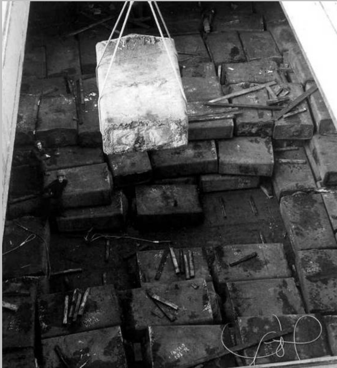
Steel slabs loaded on to wooden spacers
